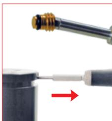
4. Hang and release the one way valve from the hole by using the one way valve removing-setting dynamometric wrench (58CD01). It would be normal some oil leak from the hole when upside down the cylinder.
