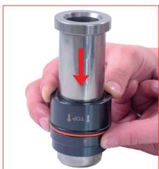
9. Slide off the cartridge from the rod. Discard the cartridge.
