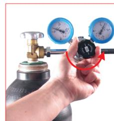
24. Adjust the required charging pressure through the regulation valve. Usually the gauge on the right display the set charging pressure. 39R... pressure reducer.
