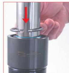
19. Position the retaining C-ring into the conical centring guide tube.
