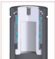
5.1. Cut off of cylinder to see the right position of the cartridge and C-ring after operation.
