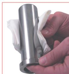
11. Carefully check and clean the piston-rod. If the piston rod shows any wear or damage do not use it again and replace it with a new one.
