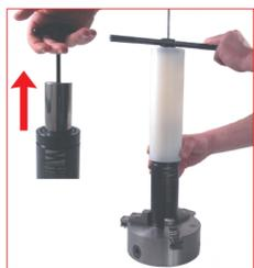
8. By using the T-handle M8 (58EM08) extract the piston-rod and the cartridge from the body (only model S500; S750). By using the proper Screw extracting device (58EV...) extract the piston-rod and the cartridge for other models.
