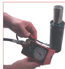
C. Connect the female quick fit on the male quick fit on the panel (39DMCPVA) and open the gas tap. For an easy and safety work carefully follow the instructions supplied with the charging unit (39DMA).
