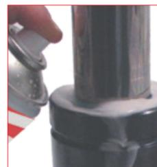
E. Use the Special Springs gas detector (39RFG) to check hose cylinders connections.
