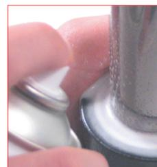
30.1. It is always recommended to check leaks on the charging port after the maintenance work and before re-using the cylinders by using the special gas detector (39RFG).
