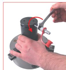
28. Unthread and release the adapter from the charging hole.
