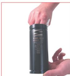
10. Carefully check and clean the cylinder body. If the body show any wear or damage do not use it again and replace it with a new one.
