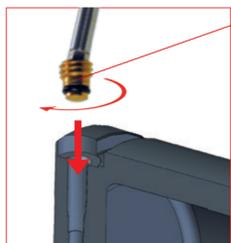
12. Position and thread the one way valve into the hole by using the appropriate special dynamometric tool already calibrated. **Torque force required maximum 0,5 Nm.** Do not exceed the maximum torque force indicated to not damage the one way valve. 58CD01 dynamometric wrench.
