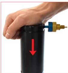
3. Be sure the pressure is completely exhausted by pressing down the piston rod into the cylinder body. Then unthread the discharging device from the discharging hole.
