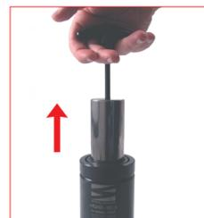
22. After threading the T-handle M8 (58EM08) into the rod head threaded hole, pull completely the unit piston-rod and bushing.
