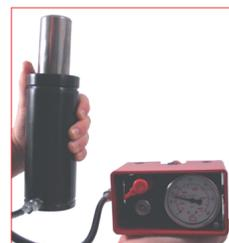
A. For charging hosed system use the proper device (39DMPCVA) to connect the control panel.
