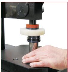
14. With the manual press (39PM02) insert the assembled bushing into the rod. Be care to position it on the right side, follow the laser print arrows on the bushing.
