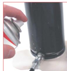
D. Use the Special Springs gas detector (39RFG) to check hose cylinders connections.
