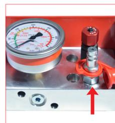
A. When required the adjusting of pressure can be easily adjusting acting/opening the discharging valve on the control panel.
