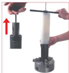
9. By using the T-handle M8 (**58EM08**) extract the piston-rod and the bushing from the rod (only model SC500B; SCF500A; SC750B; SCF750A; H/HF700A; H/HF1000A). By using the proper Screw extracting device (**58EV...**) extract the piston-rod and the bushing from the other models.
