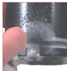
32. It is always recommended to check leaks on the charging port after the maintenance work and before re-using the cylinders by using the special gas detector. **39RFG** Special Springs gas detector.
