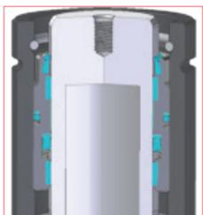
6.1. Cut off of cylinder to see the right position of the cartridge and C-ring after operation.
