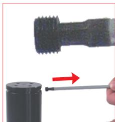
4. Unthread the valve retaining screw by using the hex key (**58CE05**). Preserve the valve retaining screw for reassembly.
