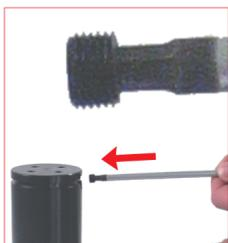
14. By using the hex key (**58CE05**) thread the one way valve retaining screw 1/8"G (**47G1/8G**). Pay attention to not tight excessively the retaining screw to avoid damage on the one way valve. **Torque force required max 1,4 Nm.**
