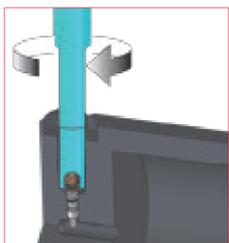
13.1. Cut off of piston-rod with the one way valve correctly positioned. Make easier the positioning by a light turning made by using the proper tool (**47ASVU**).
