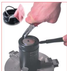
8. By using the removal C-ring (**58EAR**) and the Multipurpose clamp (**58KNIPEX**) hook up the retaining C-ring. Preserve the retaining C-ring for reassembly.
