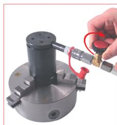
29. When directly charging through the adapter and desired pressure is reached shut off the hose and bottle valves and disconnect the the quick fit coupling. For an easy and safety work carefully follow the instructions supplied with the charging unit. **39DMCPVA** charging unit. **QDFV...** adapter for direct charging.
