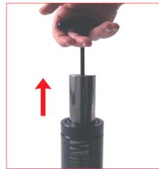
24. Manually extract the assembly piston-rod/cartridge until it rests against the C-ring. **58EM08** T-handle M8.
