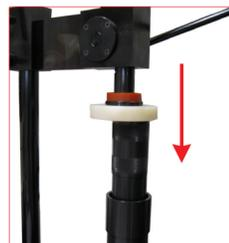
23. Insert the positioning tube in contact with the retaining C-ring, then by the manual press, press down the retaining C-ring into the groove. When the C-ring enters correctly into the groove you will hear a loud like "CLICK". **49TB...** conical centring guide tube. **39PM02A** manual press.
