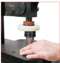
16. Manually or by using the manual press (**39PM02A**) insert the assembled bushing into the rod. Be care to position it on the right side, follow the laser print arrows on the bushing.
