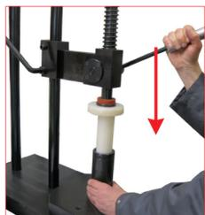
6. Position the anti scratch nylon removal tube on the cartridge (**49TN...**) then by the manual press (**39PM02A**) press all down into the body. The retaining ring is now free for an easy removal.
