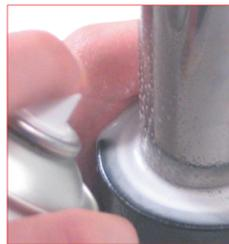
E. It is always recommended to check leaks on the upper side of the cylinders after the maintenance work and before re-using the cylinders by using the special gas detector. **39RFG** Special Springs gas detector.
