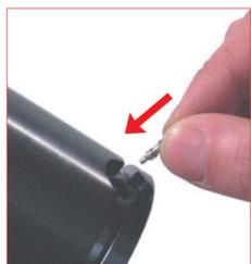
13. Carefully clean through the charging hole with an air gun, then drop the new one way valve (**59VU**) into the conical hole.
