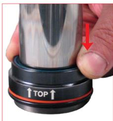
17. Slide down the assembled bushing to the piston shoulder.
