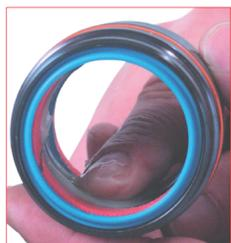
15. Take the new assembled bushing and grease inside all over by using the specific Special Springs grease compound supplied with the repair kit.
