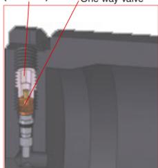
14.1. Cut off of the conical hole with the one way valve and the 1/8"G one way valve retaining screw correctly positioned.
