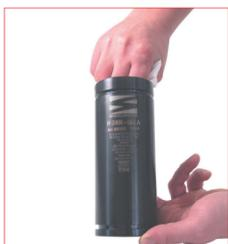
11. Carefully check and clean the cylinder body. If the cylinder body shows any damage or wear do not use it again and replace it with a new one.
