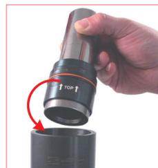
20. Set the positioning tube on the upper part of the cylinder body, then manually insert the piston-rod and the assembled bushing into the positioning tube. **49TB...** positioning tube.
