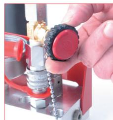
C. Connect the female quick fit on the male quick fit on the panel and open the gas tap. For an easy and safety work carefully follow the instructions supplied with the charging unit. **39DMCPVA** control panel charging unit.
