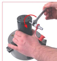
30. Unthread and release the adapter from the charging hole.
