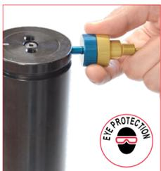
2. Thread DDS bleed device on the charging port then exhaust completely the pressure. Point away from the operator for maximum safety. **39DDS01A** for the 1/8 G port.
