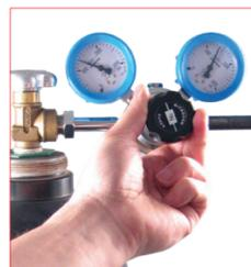
B. Adjust the required pressure on the regulation valve on the bottle. The gauge on the right will indicate the maximum allowed pressure to charge the cylinders. **39R...** pressure regulation valve.
