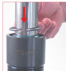
22. Position the retaining C-ring into the conical centring guide tube.
