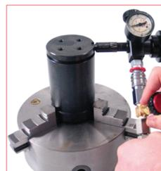
27. Select and assemble the desired charging adapter and thread it on the charging port. For an easy and safety work carefully follow the instructions supplied with the charging unit. **DO NOT** exceed the maximum pressure indicated for any specific model. **39DMA** charging unit.
