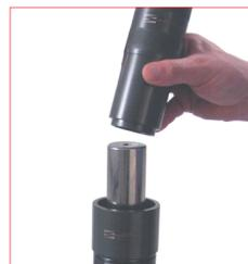
21. Insert the positioning tube over the rod in contact with the upper side of the assembled bushing, then by the manual press, press down into the cylinder body, the piston rod and the assembled bushing. **49TB...** conical centring guide tube. **39PM02A** manual press.
