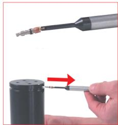
5. Hang and remove the one way valve from the conical lodging site by using the proper tool (**39EVU**).
