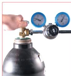
25. Check the correct assembly of the pressure regulation valve on the gas bottle, then open the main tap. The gauge on the left will indicate the bottle pressure. **39R...** pressure regulation valve.
