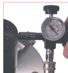
27. Select and assemble the desired charging adapter on the charging unit device (DMA), thread it on the charging hole and proceed to fill the gas on the desired pressure (Max. 150 if not different specified). Do not exceed the maximum indicated charging pressure.
