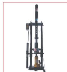
31. More precise force control can be carried out by using the digital Special Springs force test rig FT... Digital force tester IPCDIG Digital force tester
