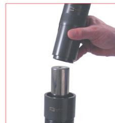
22. Insert the positioning tube (49TB...) over the rod. Carefully verify the tube is correctly rest against the top side of the assembled bushing.
