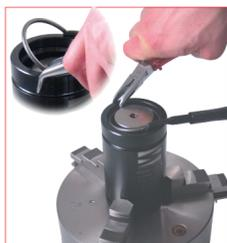
8. By using the removal C-ring (58EC) and the Multipurpose clamp (58KNIPEX) hook up the retaining C-ring. Preserve the retaining C-ring for reassembly.
