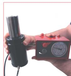
A. For charging hoses system use the proper device (DMPCVA) to connect the control panel.
