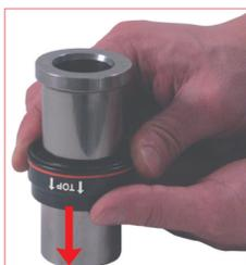
10. Then slide off the bushing from the rod and discard the bushing.
