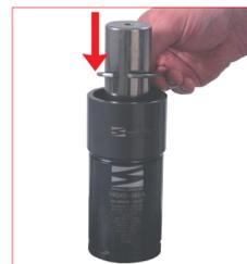
21. Then position the retaining C-ring into the assembly guiding tube.
