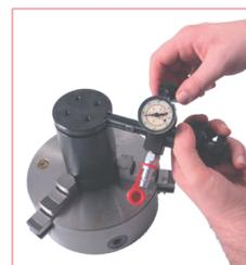
35. When required the adjusting pressure can be easily adjusted by using the main unit (DMCLA) of the Special Springs charging device. More details included with DMA instruction manual.
