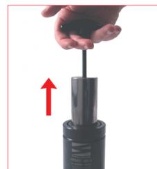
24. After threading the T-handle M8 into the rod head threaded hole, pull completely the unit piston-rod and bushing.
