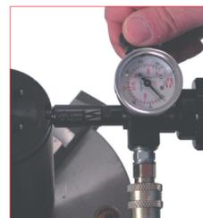
28. Wait a while for pressure stabilization, close the shut-off hose and bottle valves. Then unthread adapter from cylinder. More detail included with the DMA instruction manual.
