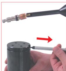
5. Hang and remove the one way valve from the conical lodging site by using the proper tool.
