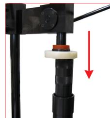
23. By using the manual press (39PM02A) act on the positioning tube to push down the retaining C-ring into its groove. When the C-ring enter into the groove you will hear a "click". Be sure the retaining C-ring is the right position into its own groove.
