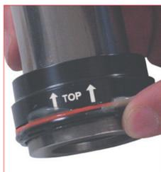
18. Grease the O-ring on the assembled bushing with the specific Special Springs grease compound supplied with the repair kit.
