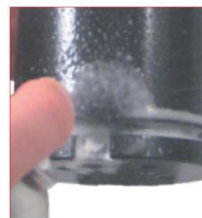
32. Use Special Springs gas detector to check leaks on valve port.
