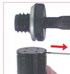
34. Thread the protective screw cap into the charging hole M6 by using the hex key (58CE03).
