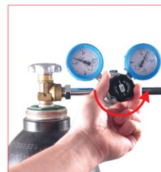
26. Adjust the required charging pressure through the regulation valve. Usually the gauge on the right display the set charging pressure. 39R... pressure regulation valve.
