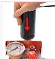
B. Be sure the pressure is completely exhausted by pressing down the piston rod into the cylinders body.
