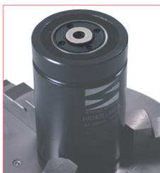
7. Clamp the cylinder into a self-centring chuck or a vise.
