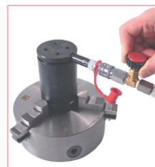
29. When charging directly through the adapter and the desired pressure is reached, shut-off hose and bottle valves and disconnect the quick fit coupling.
