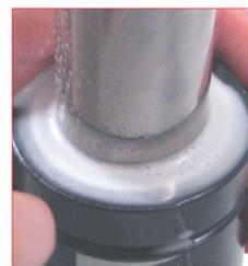
33. Use Special Springs gas detector to check leaks on the top of the body.
