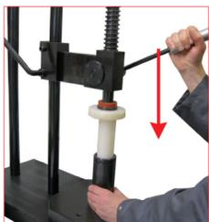
6. Position the anti scratch nylon removal tube on the cartridge then by the manual press (39PM02A) press all down into the body for about 20-25 mm. The retaining ring is now free for an easy removal.
