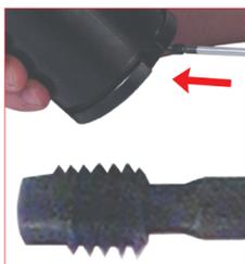
14. By using the hex key (58CE03) thread the one way valve retaining screw M6 (47GM6). Pay attention to not tight excessively the retaining screw to avoid damage on the one way valve.
