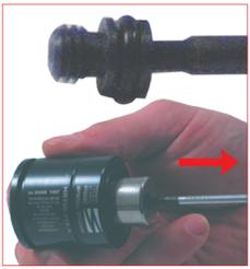
1. Remove the protective screw cap from the charging hole by using the appropriate tool. Preserve the protective screw cap for further reassembly. **58CE03** M6/3 for the M6 port.
