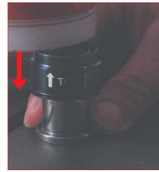
14. Manually or by using the manual press (**39PM02A**) insert the assembled bushing into the rod. Be care to position it on the right side, follow the laser print arrows on the bushing.
