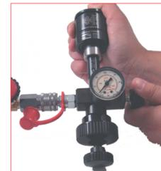
30. It is always recommended to check leaks on the charging port after the maintenance work and before re-using the cylinders by using the special gas detector. **39RFG** Special Springs gas detector.
