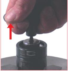
7. By using the T-handle (**58EM06**) extract the piston-rod and the bushing from the body.
