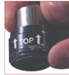
16. Grease the O-ring on the assembled bushing with the specific Special Springs grease compound supplied with the repair kit.
