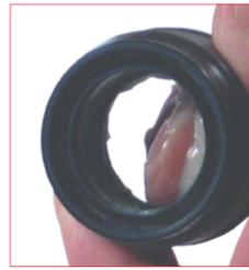
13. Take the new assembled bushing and grease inside all over by using the specific Special Springs grease compound supplied with the repair kit.
