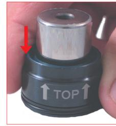
15. Slide down the assembled bushing to the piston shoulder.
