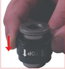
8. Slide off the bushing from the rod and discard the bushing.
