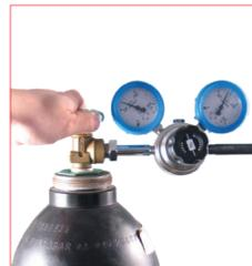
27. When directly charging through the adapter and desired pressure is reached shut off the hose and bottle valves and disconnect the quick fit coupling. For an easy and safety work carefully follow the instructions supplied with the charging unit. **39DMCPVA** charging unit. **39QDFV...** adapter for direct charging.
