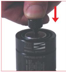
3. Be sure the pressure is completely exhausted by pressing down the piston rod into the cylinder body. Then unthread the discharging device from the discharging hole.
