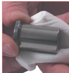
11. Carefully check and clean the piston-rod. If the piston-rod shows any damage, wear or scratch do not use it again and replace it with a new one.
