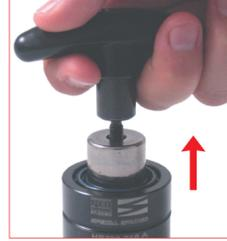
24. Adjust the required charging pressure through the regulation valve. Usually the gauge on the right display the set charging pressure. **39R...** pressure regulation valve.
