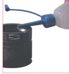
17. Lubricate inside the cylinder body with the specific Special Springs oil supplied with the repair kit. Be care to the quantity as indicated for each cylinder model.
