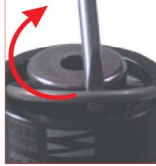
6. By using the removal C-ring hook up the retaining C-ring. Preserve the retaining C-ring for re-assembly.
