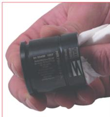
10. Carefully check and clean the cylinder body. If the cylinder body shows any damage or wear do not use it again and replace it with a new one.
