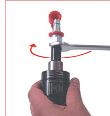
31. Thread the protective screw cap into the charging hole M6 by using the hex key (**58CE03**).
