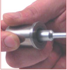
9. By using the 8 mm hex built key (**58CA08**) remove the ball retaining screw (**47VGS19A**) the ball (**59S3.17**) the spring (**59MGS**) then remove the O-ring (**50OR2004**). Preserve the spring and the ball for reassembly.
