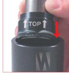
21. By using the manual press (**39PM02A**) act on the positioning tube to push down the retaining C-ring into its groove. When the C-ring enter into the groove you will hear a "click". Be sure the retaining C-ring is the right position into its own groove.
