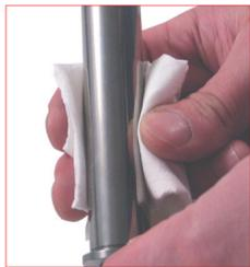
12. Carefully check and clean the piston-rod. If the piston-rod shows any damage, wear or scratch do not use it again and replace it with a new one.
