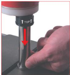
17. Manually or by using the manual press (39PM02A) insert the assembled bushing into the rod. Be care to position it on the right side, follow the laser print arrows on the bushing.
