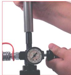
29. Reached and stabilized the desired pressure, for an easy and safety work carefully follow the instructions supplied with the charging unit.
