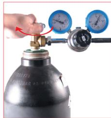
26. Check the correct assembly of the pressure regulation valve on the gas bottle, then open the main tap. The gauge on the left will indicate the bottle pressure.
