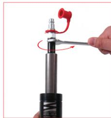
31. Unthread and release the adapter from the charging hole.
