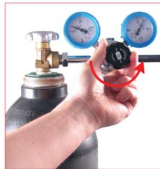
27. Adjust the required maximum pressure through the regulation valve. The gauge on the right will indicate the maximum allowed pressure to charge the cylinder.
