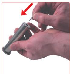
13. Carefully clean through the charging hole with an air gun, then drop the new one way valve into the conical hole.
