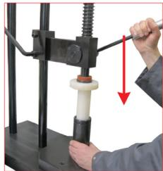
6. Position the anti scratch nylon removal tube on the cartridge (49TN...) then by the manual press (39PM02A) press all down into the body for about 20-25 mm. The retaining ring is now free for an easy removal.
