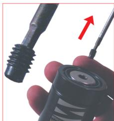
4. Unthread the valve retaining screw by using the hex key (58CE03). Preserve the valve retaining screw for reassembly.
