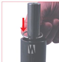
23. Position the retaining C-ring into the conical centring guide tube.
