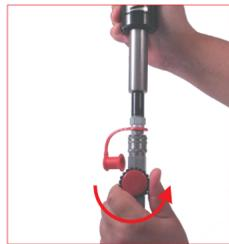
30. When directly charging through the adapter and desired pressure is reached shut off the hose and bottle valves and disconnect the the quick fit coupling. For an easy and safety work carefully follow the instructions supplied with the charging unit.
