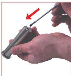
15. By using the hex key (58CE03) thread the one way valve retaining screw M6 (47GM6). Pay attention to not tight excessively the retaining screw to avoid damage on the one way valve.
