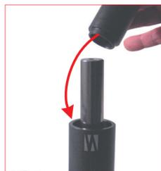
22. Insert the positioning tube over the rod in contact with the upper side of the assembled bushing, then by the manual press, press down into the cylinder body, the piston rod and the assembled bushing.
