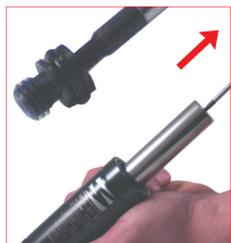
1. Remove the protective screw cap from the charging hole M6 by using the hex key (58CE03). Preserve the screw cap from reassembly.
