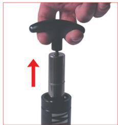
9. By using the T-handle (58EM06) extract the piston-rod and the bushing from the body.
