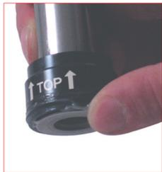
19. Grease the O-ring on the assembled bushing with the specific Special Springs grease compound supplied with the repair kit.
