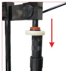
24. Insert the positioning tube in contact with the retaining C-ring, then by the manual press, press down the retaining C-ring into the groove. When the C-ring enter correctly into the groove you will hear a loud like "CLICK".
