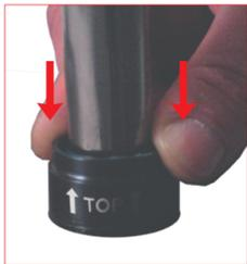
18. Slide down the assembled bushing to the piston shoulder.
