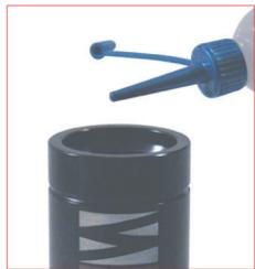
20. Lubricate inside the cylinder body with the specific Special Springs oil supplied with the repair kit. Be care to the quantity as indicated for each cylinder model.
