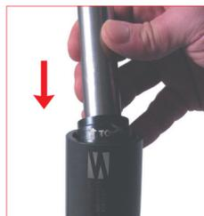
21. Set the positioning tube on the upper part of the cylinder body, then manually insert the piston-rod and the assembled bushing into the positioning tube.
