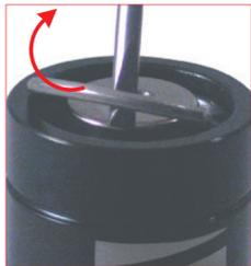
8. By using the removal C-ring (58EC) hook up the retaining C-ring. Preserve the retaining C-ring for reassembly.
