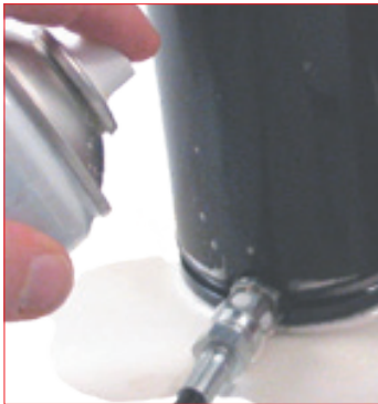
D. It is always recommended to check leaks on all connection to and from the gas spring by using the gas detector.
