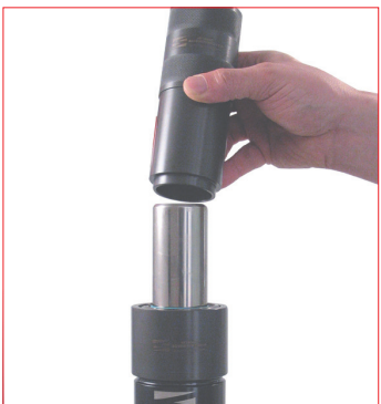
26. Insert the positioning tube over the rod in contact with the upper side of the assembled bushing, then by the manual press, press down into the gas spring body, the piston rod and the assembled bushing. 49TP... positioning tube. 39PM02A manual press.
