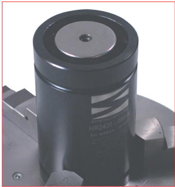
12. Position and clamp the gas spring into a self-centring chuck or a vice.
