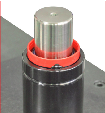
40. Direct the V-shaped discharging section, as shown in the image. Place the Over Stroke Marker by aligning the indicator tooth with the discharging grooves.
