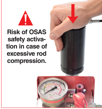
B. Make sure that no gas remains inside the gas springs connected to the system by PARTIALLY compressing the rods into the bodies.
