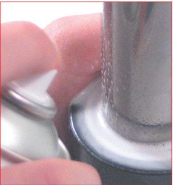
E. It is always recommended to check leaks on the upper side of the gas springs after the maintenance work and before re-using the gas springs by using the gas detector.
