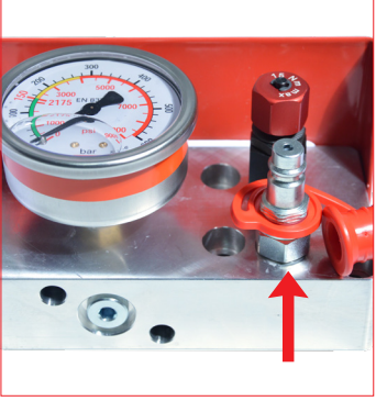
A. After positioning and hosing all the gas springs, proceed through the quick fit device through the control panel for charging all the gas springs. Make sure that the discharging valve is closed properly (15 Nm). 39DMCPVA control panel charging unit.
