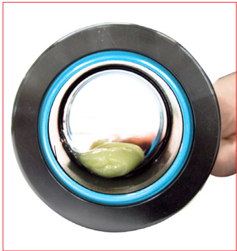
20. Lubricate all the installed components into the assembled bush with the Special Springs grease.
