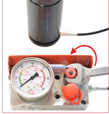
A. To exhaust pressure of hosed cylinders open the discharging valve on the control panel.
