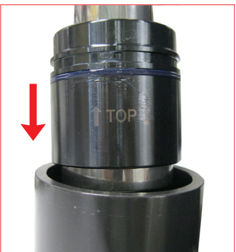
25. Set the positioning tube on the upper part of the gas spring body, then manually insert the piston-rod and the assembled bushing into the positioning tube. 49TC...positioning tube.
