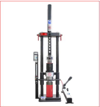
36. More precise force control can be carried out by using the digital force testing rigs. FT... Digital force tester
