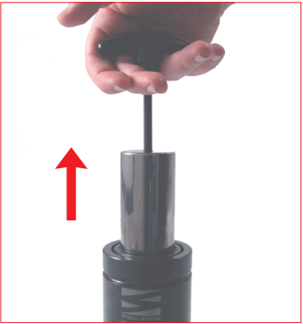
29. Manually extract the assembly piston-rod/bush until it rests against the C-ring. 58EM06A T-handle M6 58EM08A T-handle M8.
