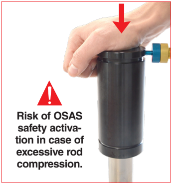
9. Make sure that no gas remains inside the gas spring by PARTIALLY compressing the rod into the body, then remove the discharging device from the charging hole.
