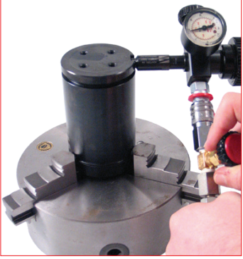
32. Select and assemble the desired charging adapter and thread it on the charging port. For an easy and safe operation carefully follow the instructions supplied with the charging unit. Do NOT exceed the maximum pressure indicated for any specific model 39DMA charging unit.
