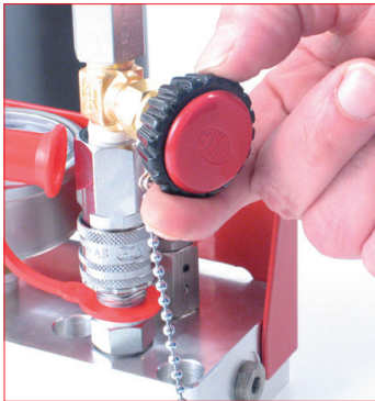
C. Connect the female quick fit on the male quick fit on the panel and open the gas tap. For an easy and safe work carefully follow the instructions supplied with the charging unit. 39DMCPVA control panel charging unit.
