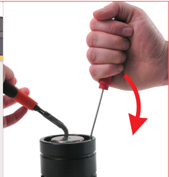
13. By inserting the screwdriver on the appropriate discharging groove, between the retaining ring and the body border, remove the ring as indicated. Use the flat screwdriver 2,5 x 75.
