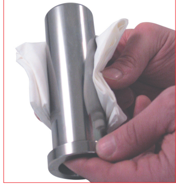
17. Carefully check and clean the piston-rod. If the piston rod shows any damage, wear or scratch do NOT use it again and replace it with a new one.
