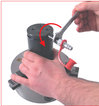
35. Thread and relase the adapter from the charging hole.
