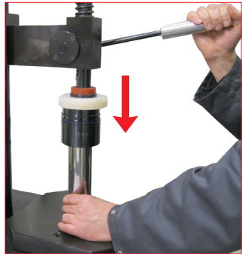
21. With the manual press (39PM02A) insert the assembled bush into the rod. Pay attention to position it on the right side, follow the laser print arrows on the bush. (↑TOP)
