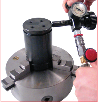
33. Once reached and stabilized the desired pressure, for an easy and safe operation carefully follow the instructions supplied with the charging unit. 39DMA charging unit.
