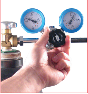
B. Adjust the required pressure on the regulation valve on the bottle. The gauge on the right will indicate the maximum allowed pressure to charge the gas springs. 39RHP... pressure reducer.
