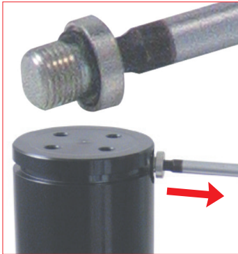
39. Thread the protective screw into the charging hole by using the appropriate tool. 58CE05 for 1/8G charging port 58CE03 for M6 charging port.
