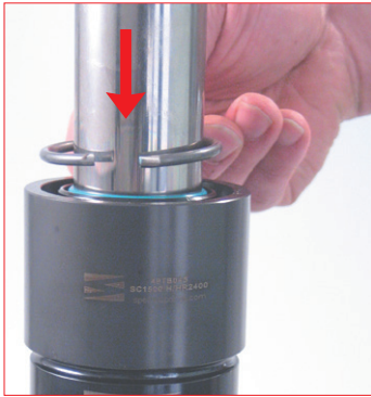
27. Position the retaining C-ring into the conical centring guide tube.
