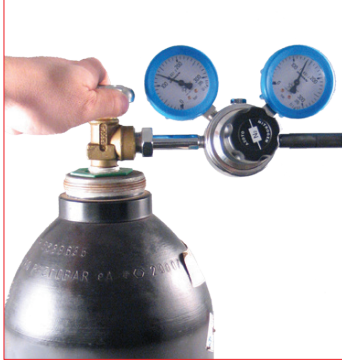
30. Check the correct assembly of the pressure regulation valve on the gas bottle, then open the main tap. The gauge on the left will indicate the bottle pressure. 39RHP... pressure reducer.
