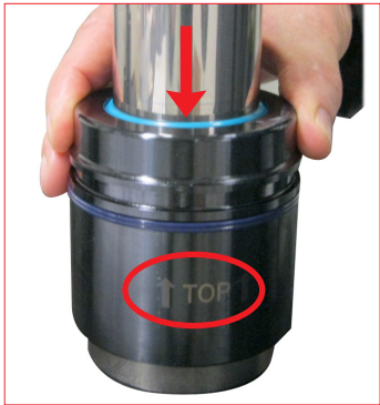
22. Slide down the assembled bush to the piston shoulder.
