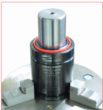
1. Position and clamp the gas spring into a selfcentring chuck or a vice.
