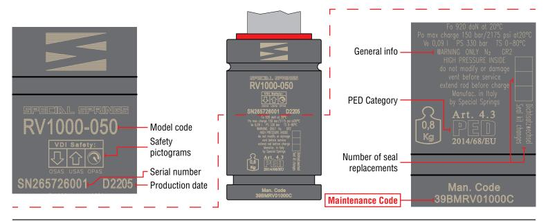
To order a maintenance kit, you are requested to communicate the Man. Code, generally marked on the bottom of the body, to your Special Springs supplier.
