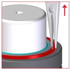
6- Remove the broken Over Stroke Marker ring from its with a pliers.
