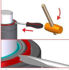
5- By using a rubber mallet, hit the flathead screwdriver to break the OSM ring halfway.
