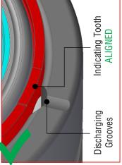
2- On the upper side of the cylinder's body, find the indicating tooth on the OSM ring and the discharging grooves.
