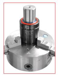
1- Secure the cylinder onto a self-centring chuck or a vice.
