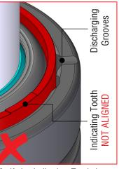
3- If the Indicating Tooth is not aligned with the discharging grooves, reposition it manually.
