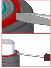
4- Positiontheflatheadscrewdriver at the center of the discharging grooves and keep it in contact with the Over Stroke Marker ring.
