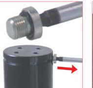
**39.** Thread the protective screw into the charging hole by using the appro-58CE05 for 1/8G charging port.
