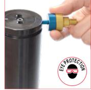
8. Thread DDS discharging device on the charging port then exhaust completely the pressure. Point away from the operator for maximum safety. 39DDS01A BLUE side for M6 hole GOLD side for 1/8"G hole
