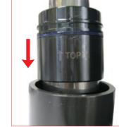
25. Set the positioning tube on the upper part of the cylinder body, then manually insert the piston-rod and the assembled bushing into the position-
