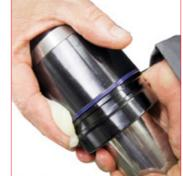
23. Grease the external seal on the assembled bush with the specific Special Springs grease.
