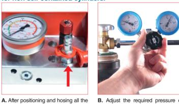
B. Adiust the required pressure on the regulation valve on the bottle. The gauge on the right will indicate the maximum allowed pressure to charge the cylinders. 39R... pressure reducer.
