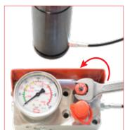
A. To exhaust pressure of hosed cilynders open the discharging valve on the control panel
