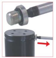
7. Remove the charging plug from the charging hole by using the appropriate tool. Preserve the charging plug for further
