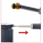
10. Hang and release the one way valve from the hole by using the appropriate tool. Some oil leaks may occur when cylinder is upside down. 58CD01 one way valve removingsetting dynamometric wrench.
