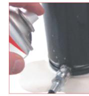
**D.** It is always recommended to check leaks on all connection to and from the cylinder by using the special gas
