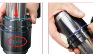
22. Slide down the assembled bush to the piston shoulder
