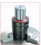
1. Position and clamp the cylinder into a self - centring chuck or a vice .
