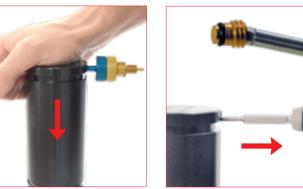
9. Be sure the pressure is completley exhauted by pressing down the piston rod into the cylinder body. Then unthread the discharging device from the discharging hole.
