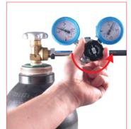
31. Adjust the required maximum pressure trought the regulation valve. The gauge on the right will indicate the maximum allowed pressure to charge the cylinder.
