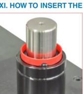
40. Direct the V-shaped discharging section, as shown in the image. Place the Over Stroke Marker by aligning the indicator tooth with the discharging grooves.
