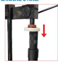
28. Insert the positioning tube in contact with the retaining C-ring , then by
