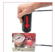
B. Be sure the pressure is completley exhausted by pressing down the piston rod into the cilynders body.
