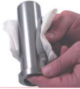
17. Carefully check and clean the piston-rod. If the piston rod shows any damage, wear or scratch do not use it again and replace it with a new one.
