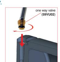
19. Position and thread the one way valve into the hole by using the appropriate special dynamometric tool already calibrated. Torque force required maximum 0.6 Nm. Do not exceed the maximum torque force indicated to not damage the one way
