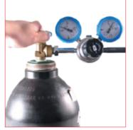
30. Check the correct assembly of the pressure regulation valve on the gas bottle, then open the main tap. The gauge on the left will indicate the
