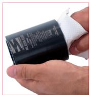
15. Carefully check and clean the cylinder body, blowing inside pressurized air to remove residuals from the grooves. If the body show any wear or damage DO NOT use it again and replace it with a new one.
