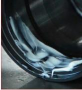
25. Lubricate the bottom grooves using the Special Springs grease. **590GRASSO** Special Springs grease
