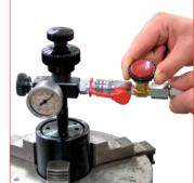
charging adapter and thread it on the charging port. For an easy and safe operation carefully follow the instruc-tions supplied with the charging unit. DO NOT exceed the maximum pressure indicated for any specific model. 39DMA charging unit.
