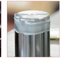
26. Lubricate the top of the rod using the Special Springs grease. 590GRASSO Special Springs grease
