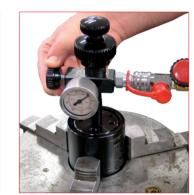
33. Check the correct assembly of 34. Adjust the required maximum 35. Select and assemble the desired 36. Once reached and stabilized the desired pressure, for an easy and safe operation carefully follow the instructions supplied with the charging unit.
