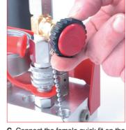
C. Connect the female quick fit on the male quick fit on the panel and open the gas tap. For an easy and safe operation carefully follow the instructions supplied with the charging unit. 39DMCPVA control panel charging
