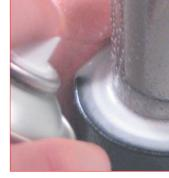
E. It is always recommended to check leaks on the upper side of the cylinders after the maintenance work and before re-using the cylinders by using the special gas detector.
