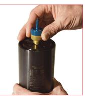
2. Thread DDS discharging device on the charging port then exhaust completely the pressure. Point away from the operator for maximum safety. 39DDS01A BLUE side for M6 hole GOLD side for 1/8"G hole
