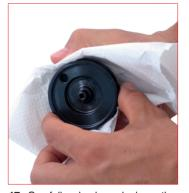
17. Carefully check and clean the bottom base, blowing inside pressurized air to remove residuals from the dual-ring groove and charging port. If the bottom base shows any wear or damage DO NOT use it again and replace it with a new one.
