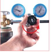
pressure trought the regulation valve. The gauge on the right will indicate the maximum allowed pressure to charge the cylinder. 39R... pressure regulation valve.
