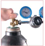
the pressure regulation valve on the gas bottle, then open the main tap. The gauge on the left will indicate the bottle pressure. **39R...** pressure regulation valve.
