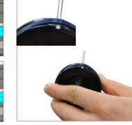
**14.** Remove the seal from the bottom base without scratching the internal
