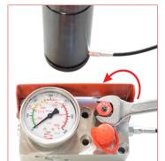
A. To exhaust pressure of linked cilynders open the discharging valve on the control panel.
