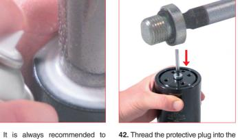
41. It is always recommended to check leaks on the upper side of the cylinders after the maintenance work and before re-using the cylinders by using the special gas detector.
