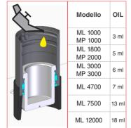
28. Put inside the cylinder the lubricating oil in the correct quantity as mentioned above
