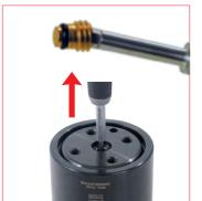
4. Unscrew and remove the one way valve from the hole by using the appropriate tool. It would be normal some oil leak from the hole when upside down the cylinder. 58CD01 Torque wrench for one way
