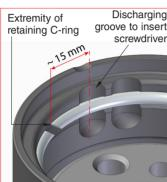
8. Position the extremity of the retaining ring at about 15 mm from the groove centre.
