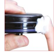
24. Lubrificate all the installed elements using the Special Spring grease. **590GRASSO** Special Springs grease
