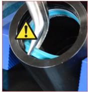
22. Install in the same groove the gas seal. If necessary, use the pliers avoiding damaging the lips of the gas **58KNIPEX** pliers
