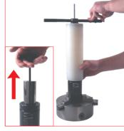
**14.** Extract the rod + the bush using the manual extractor (58EM ...) or the suitable screw extractor (58UT ...).
