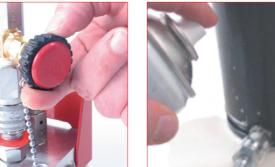
C. Connect the female quick fit on the male quick fit on the panel and open the gas tap. For an easy and safety work carefully follow the instructions supplied with the charging unit.
