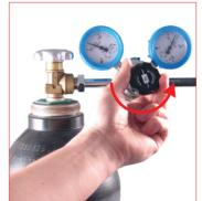
31. Adjust the required maximum pressure trought the regulation valve. The gauge on the right will indicate the maximum allowed pressure to charge the gas spring. 39RHP... pressure reducer.
