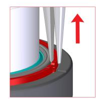
6. Remove the broken Over Stroke Marker (OSM) ring from its location with a pliers. Clean any residual mate-
