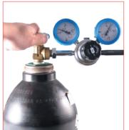
30. Check the correct assembly of the pressure regulation valve on the gas bottle, then open the main tap. The gauge on the left will indicate the bottle pressure.
