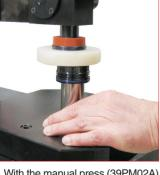
21. With the manual press (39PM02A) insert the assembled bush into the rod. Pay attention to position it on the right side, follow the laser print arrows on the bush. (**†TOP**)
