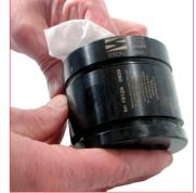
**16.** Carefully check and clean the gas spring body. If the body show any wear or damage do not use it again and replace it with a new one.
