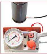
A. To exhaust pressure of hosed cilynders open the discharging valve on the control panel.
