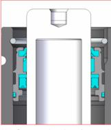
11.1. Cross section view of gas spring to see the right position of the bush and C-ring after operation.
