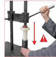
11. Position the anti scratch nylon removal tube (49TN...) on the bush then by the manual press (39PM02A) press all down into the body. The retaining ring is now free for an easy removal. A Risk of OSAS safety activation in case of excessive rod compression A
