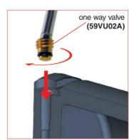
19. Position and thread the one way valve into the hole by using the appropriate special dynamometric tool already calibrated. Torque force required maximum 0,6 Nm. Do not exceed the maximum torque force indicated to not damage the one way 58CD01 dynamometric wrench.
