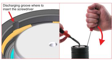
13. By inserting the screwdriver on the appropriate discharging groove, between the retaining ring and the body border, remove the ring as indicated. Use the pliers (58KNIPEX) to avoid that the ring comes out sharply. Use the flat screwdriver 2,5 x 75.
