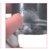
check leaks on the charging port after the maintenance work and before re-using the gas springs by using the gas detector.
