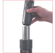
26. Insert the positioning tube over the rod in contact with the upper side of the assembled bushing, then by the manual press, press down into the gas spring body, the piston rod and the assembled bushing. 49TP... tubo di posizionamento
