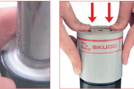
FOR RS GAS SPRINGS ONLY. Manually reassembly the protective SKUDO on the rod. It would be required a light pressure to correctly position it. When the protective SKUDO cap enter correctly into the groove you will hear a sound like "CLICK".
