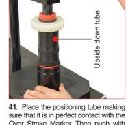
Over Stroke Marker. Then push with the press and place the Over Stroke Marker ring into its location. The correct positioning will produce a sound like a "CLICK" 49TP.... Positioning tube. 39PM02A Manual press.
