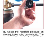
gauge on the right will indicate the maximum allowed pressure to charge the gas springs. 39RHP... pressure reducer.
