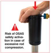
9. Make sure that no gas remains inside the gas spring by A PARTIALLY compressing the rod into the body, then remove the discharging device from the charging hole.
