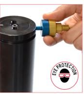
8. Thread DDS discharging device on the charging port then exhaust completely the pressure. Point away from the operator for maximum safety. 39DDS01A BLUE side for M6 hole GOLD side for 1/8"G hole
