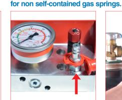
**A.** After positioning and hosing all the gas springs, proceed through the quick fit device trough the control panel for charging all the gas springs. Make sure that the discharging valve is closed properly (15 Nm). 39DMCPVA control panel charging
