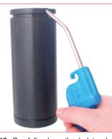
18. Carefully clean the lodging hole of the valve with compressed air and then position the new one way valve supplied along with the maintenance kit. Pay attention to its right position.
