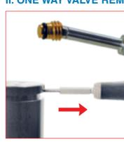
4. Hang and release the one way valve from the hole by using the one way valve removing-setting dynamometric wrench (58CD01). It would be normal some oil leak from the hole when upside down the cylinder.
