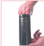
10. Carefully check and clean the 11. Carefully check and clean the cylinder body. If the body show any wear or damage do not use it again and replace it with a new one.
