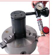
32. When required the adjusting pressure remove the protective screw cap into the charging hole 1/8" by using the hex key (58CE05), then use the main unit (39DMCILA) of the Special Springs charging device. More details included with (39DMCILA) instruction manual.
