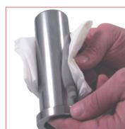
piston-rod. If the piston rod shows anv damage, wear or scratch do not use it
