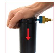
3. Be sure the pressure is completley exhauted by pressing down the piston rod into the cylinder body. Then unthread the discharging device from the discharging hole.
