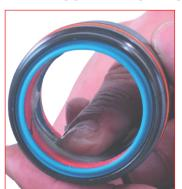
13. Lubrificate all the installed components into the assembled bushing with the Special Springs grease.
