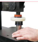
14. With the manual press (39PM02) insert the assembled bushing into the rod.
