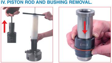
9. Slide off the cartridge from the rod. Discard the cartridge. (58EM08) extract the piston-rod and the cartridge from the body (only model S500; S750). By using the
