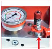
A. When required the adjusting of pressure can be easly adjusting acting/opening the discherging valve on the control panel.
