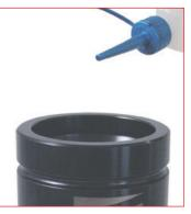
17. Lubrificate inside the cylinder body with the specific Special Springs oil supplied with the repair kit. Be care to the quantity as indicated for each cylinder model.
