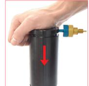
3. Be sure the pressure is completley exhauted by pressing down the piston rod into the cylinder body. Then unthread the discarging device from the discarging hole.
