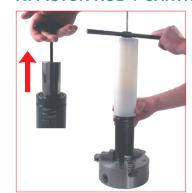
9. By using the T-handle M8 (58EM08) 10. Then slide off the bushing from extract the piston-rod and the bushing from the body (only model SC500B; SCF500A;SC750B;SCF750A;H/ HF700A;H/HF1000A). By using the proper Screw extracting device (58EV...) extract the piston-rod and the bushing from the oder models.
