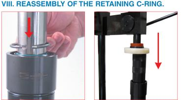
23. Insert the positioning tube in contact with the retaining C-ring, then by the manual press, press down the retaining C-ring into the groove. When
