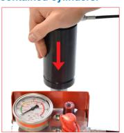
**B.** Be sure the pressure is completley exhausted by pressing down the pis-
