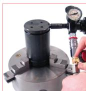
27. Select and assemble the desired charging adapter and thread it on the charging port. For an easy and safety work carefully follow the instructions supplied with the charging unit. DO NOT exceed the maximum pres-
