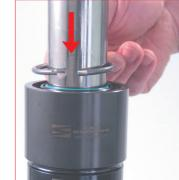
22. Position the retaining C-ring into the conical centring guide tube.
