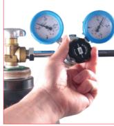
**B.** Adjust the required pressure on the regulation valve on the bottle. The gauge on the right will indicate the maximum allowed pressure to charge the cylinders.
