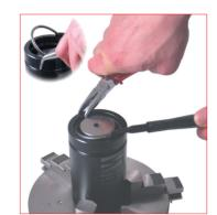
8. By using the removal C-ring (58EAR) and the Multipurpose clamp (58KNIPEX) hook up the retaining C-ring.
