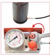
A. To exhaust pressure of hosed cilynders open the discharging valve on the control panel
