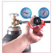
26. Adjust the required maximum pressure trought the regulation valve. The gauge on the right will indicate the maximum allowed pressure to charge the cylinder.
