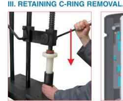
6. Position the anti scratch nylon removal tube on the cartridge (49TN...) then by the manual press (39PM02A) press all down into the body. The retaining ring is now free for an easy removal.
