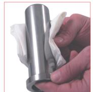
12. Carefully check and clean the piston-rod. If the piston-rod shows any damage, wear or scratch do not use it again and replace it with a new one.
