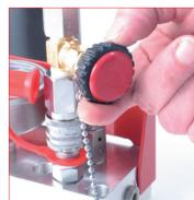
C. Connect the female quick fit on the male guick fit on the panel and open the gas tap. For an easy and safety work carefully follow the instructions supplied with the charging unit. 39DMCPVA control panel charging
