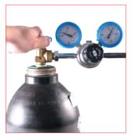
25. Check the correct assembly of the pressare regulation valve on the gas bottle, then open the main tap. The gauge on the left will indicate the
