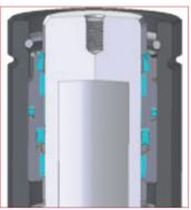
**6.1.** Cut off of cylinder to see the right position of the cartridge and C-ring
