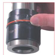
18. Grease the O-ring on the assembled bushing with the specific Special Springs grease compound supplied with the repair kit.
