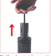
24. Manually extract the assembly piston-rod/cartridge untill it rests against the C-ring 58EM08 T-handle M8.
