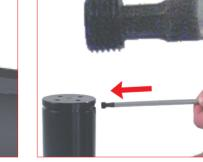
14. By using the hex key (58CE05) thread the one way valve retaining screw 1/8"G (47G1/8G). Pay attention to not tight exessively the retaining screw to avoid damage on the one way valve.
