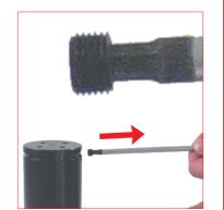
4. Unthread the valve retaining screw by using the hex key (58CE05). Preserve the valve retaining screw for reassembly.
