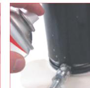
D. It is always recommended to check leaks on all connection to and from the cylinder by using the special gas
