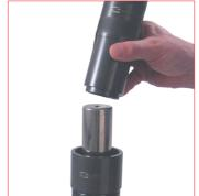
21. Insert the positioning tube over the rod in contact with the upper side of the assembled bushing, then by the manual press, press down into the cylinder body, the piston rod and the assembled bushing.
