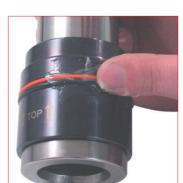
17. Slide down the assembled bushing to the piston shoulder
