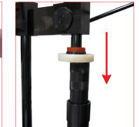
23. By using the manual press (39PM02A) act on the positioning tube to push down the retaining C-ring into it's groove. When the C-ring enter into the groove you will hear a "click".
