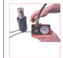
C. Charge the system to desired pressure. More details included with DMA instruction manual.
