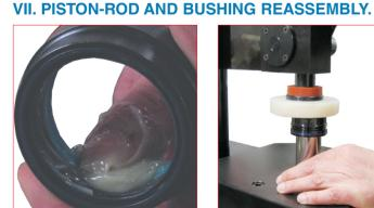
15. Take the new assembled bushing and grease inside all over by using the specific Special Springs grease compound supplied with the repair kit.
