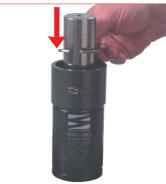
21. Then position the retaining C-ring into the assembly guiding tube.
