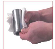
12. Carefully check and clean the piston-rod. If the piston-rod shows any damage, wear or scratch do not use it again and replace it with a new one.
