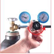
26. Adjust the required charging pressure trought the regulation valve. Usually the gauge on the right display the set charging pressure. 39R... pressure regulation valve.
