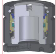
**6.1.** Cut off of the cylinder to see the right position of the cartridge and C-ring after operation #6.
