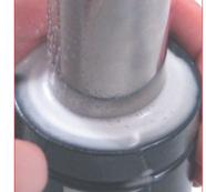
33. Use Special Springs gas detector to check leaks on the top of the body.
