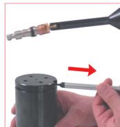
5. Hang and remove the one way valve from the conical lodging site by using the proper tool.
