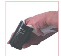
11. Carefully check and clean the cylinder body. If the cylinder body shows any damage or wear do not use it again and replace it with a new one.
