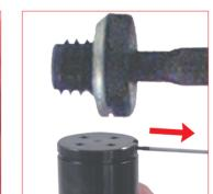
34. Thread the protective screw cap into the charging hole M6 by using the hex key (58CE03).
