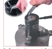
8. By using the removal C-ring (58EC) and the Multipurpose clamp (58KNIPEX) hook up the retaining C-ring. Preserve the retaining C-ring for reas-
