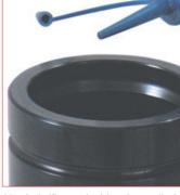
19. Lubrificate inside the cylinder body with the specific Special Springs oil supplied with the repair kit. Be care to the quantity as indicated for each cylinder model.
