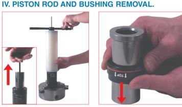
10. Then slide off the bushing from the rod and discard the bushing
