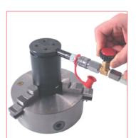
29. When charging directly throught 30. Unthread the adapter from the the adapter and the desired pressure is reached, shut-off hose and bottle valves and disconnect the quick fit coupling.
