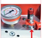
A. When required the adjusting of pressure can be easly adjusting acting/opening the discherging valve on the control panel.
