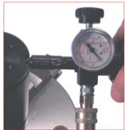
charging adapter on the charging unit tion, close the shut-off hose and bottle device (DMA), thread it on the charging hole and proceed to fill the gas on the desired pressure (Max. 150 if not different specified). Do not exceed the maximum indicated instruction manual.
