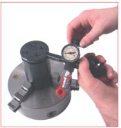
35. When required the adjusting pressure can be easly adjusted by using the main unit (DMCILA) of the Special Springs charging device. More details included with **DMA**instruction manual.
