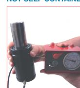
A. For charging hosed system use the proper device (DMPCVA) to connect the control panel.
