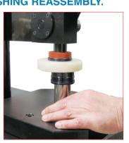
**16.** Manually or by using the manual press (39PM02A) insert the assembled bushing into the rod. Be care to position it on the right side, follow the laser print arrows on the bushing.
