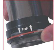
18. Grease the O-ring on the assembled bushing with the specific Special Springs grease compound supplied with the repair kit.
