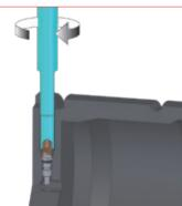
13.1 Cut off of piston-rod with the one way valve correctley positioned Make easier the positioning by a light turning made by using the proper tool (47ASVU).
