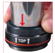
17. Slide down the assembled bushing to the piston shoulder
