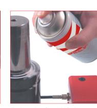
E. Use the Special Springs gas detector to check top side of cylinders body and bushing.
