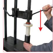
6. Position the anti scratch nylon removal tube on the cartridge then by the manual press (39PM02A) press all down into the body for about 20-25 mm. The retaining ring is now free for an easy removal.
