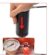
B. Be sure the pressure is completley exhausted by pressing down the piston rod into the cilynders body.
