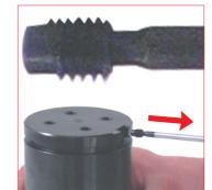
4. Unthread the valve retaining screw by using the hex key (58CE03). Preserve the valve retaining screw for reassembly.
