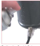
D. Use the Special Springs gas detector to check hose cylinders connections.
