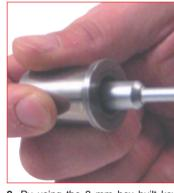
9. By using the 8 mm hex built key 9.1. Cut off of the valve assembly 9.2. Cut off of after the ball retaining 9.3. Cut off of after the spring remov-(58CA08) remove the ball retaining screw (47VGSMC19A) the ball (59S3.17) the spring (59MGS) then remove the O-ring (50OR2004). Preserve the spring and the ball for reassembly.
