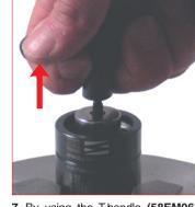
extract the piston-rod and the bushing from the body.
