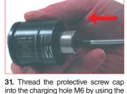
into the charging hole M6 by using the hex key (58CE03).
