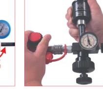
25. Select and assemble the desired charging adapter on the charging unit device (39DMA), thread it on the charging hole and proceed to fill the gas on the desired pressure (Max. 150 if not different specified). Do not exceed the maximum indicated charging pressure.
