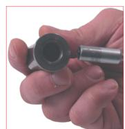
12. Carefully clean through the charging hole with an air gun, then drop the new valve components (59VU) into the conical hole.
