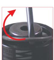
6. By using the removal C-ring hook up the retaining C-ring.
