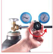
24. Adjust the required charging pressure trought the regulation valve. Usually the gauge on the right display the set charging pressure. **39R...** pressure regulation valve.
