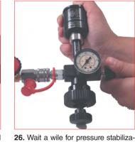
tion, close the shut-off hose and bottle Then unthread adapter from cylinder. More detail included with the 39DMA instruction manual.
