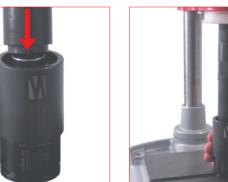
20. Insert the positioning tube (49TB...) over the rod. Carefully verify the tube is correctly rest against the top side of the assembled bushing.
