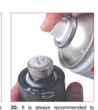
check leaks on the charging port after the maintenance work and before re-using the cylinders by using the special gas detector. 39RFG Special Springs gas detector.
