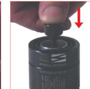
3. Be sure the pressure is completley exhauted by pressing down the piston rod into the cylinder body. Then unthread the discarging device from the discarging hole.
