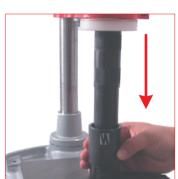
21. By using the manual press (39PM02A) act on the positioning tube to push down the retaining C-ring into it's groove. When the C-ring enter into the groove you will hear a "click". Be sure the retaining C-ring is the right position into its own groove.
