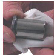
11. Carefully check and clean the piston-rod. If the piston-rod shows any damage, wear or scratch do not use it again and replace it with a new one.
