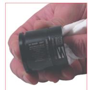
10. Carefully check and clean the cylinder body. If the cylinder body shows any damage or wear do not use it again and replace it with a new one.
