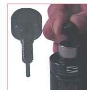
2. Thread DDS bleed device on the charging port then exhaust completely the pressure. Point away from the operator for maximum safety. DDS-M6/1 for the M6 port.
