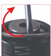
17. Lubrificate inside the cylinder body with the specific Special Springs oil supplied with the repair kit.
