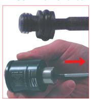
1. Remove the protective screw cap from the charging hole by using the appropriate tool Preserve the the protective screw cap for further reassembly. 58CE03 M6/3 for the M6 port.
