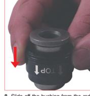
7. By using the T-handle (58EM06) 8. Slide off the bushing from the rod and discard the bushing.
