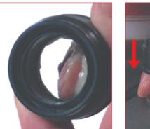
13. Take the new assembled bushing 14. Manually or by using the manual and grease inside all over by using press (39PM02A) insert the assemthe specific Special Springs grease bled bushing into the rod. Be care to position it on the right side, compound supplied with the repair kit. follow the laser print arrows on the bushing.
