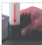
4. Position the anti scratch nylon removal tube on the cartridge (49TN...) then by the manual press (39PM02A) press all down into the body. The retaining ring is now free for an easy removal.
