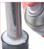
34. It is always recommended to check leaks on the upper side of the cylinders after the maintenance work and before re-using the cylinders by using the special gas detector. 39RFG Special Springs gas detector.
