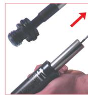
**1.** Remove the protective screw cap from the charging hole M6 by using the hex key (58CE03). Preserve the screw cap from reassembly.
