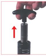
9. By using the T-handle (58EM06) 10. Then slide off the bushing from extract the piston-rod and the bushing
