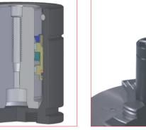
6.1. Cut of the cylinder to see the right 7. Clamp the cylinder into a selfposition of the cartridge and C-ring centring chuck or a wise. after operation #6.
