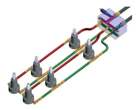
Using same-length connectors (be they of the flexible or rigid type) between the cylinders and the distribution unit guarantees the simultaneous return of the rods during the release phase of the cylinder block.
