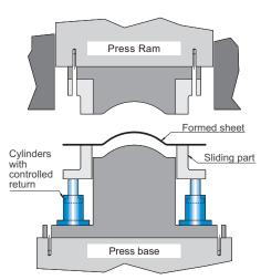
BLANK HOLDER RETURN WITH CYLINDER EXTENSION AND PRESS AT TDC
