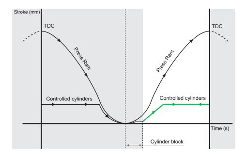
During the return phase of the press 1, a signal from the press command unit (angular position of the press shaft corresponding to a given position of the mobile slide) enables the operator to switch on the electrical distributor 9 so as to make the fluid flow through the return circuit of the cylinders.
