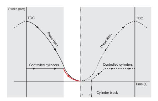
The Ram of the press 1 starts going down; the cylinder rods 2 compress and the fluid contained inside the cylinders flows through the retention valve 4 towards the pressure-reducing valve 6, which generates a counter-pressure, i. e. a contrasting force. This force may be either constant, increasing or decreasing over the whole extent of the stroke. The fluid pumped by the command unit 12 goes on flowing through the circuit of the air-oil exchanger 7.
